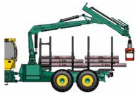
Quick-change twin stanchion for 2 x 2 or 2 x 2.5 m wood (not for 805F short version)
